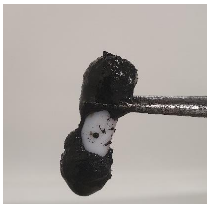
Figure 49: Fe caught by the magnetic stirrer at -1.15 V during the deposition.
