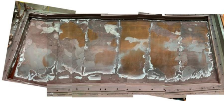
Figure 9: top view of the cathode covered by the fragmented iron produced during the trial carried out on April 22.
