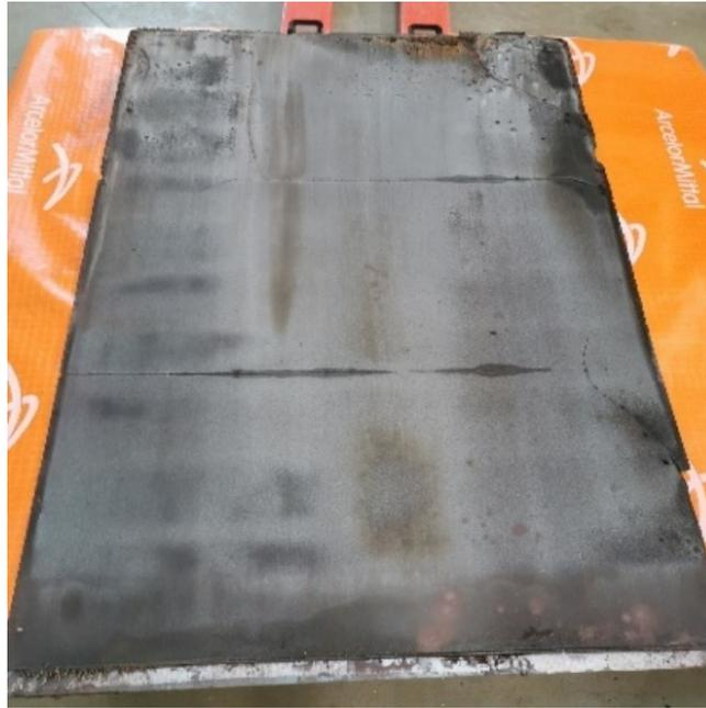
Figure 10: Iron plate produced on the Siderwin pilot with the reduced cathode (15 kg).
