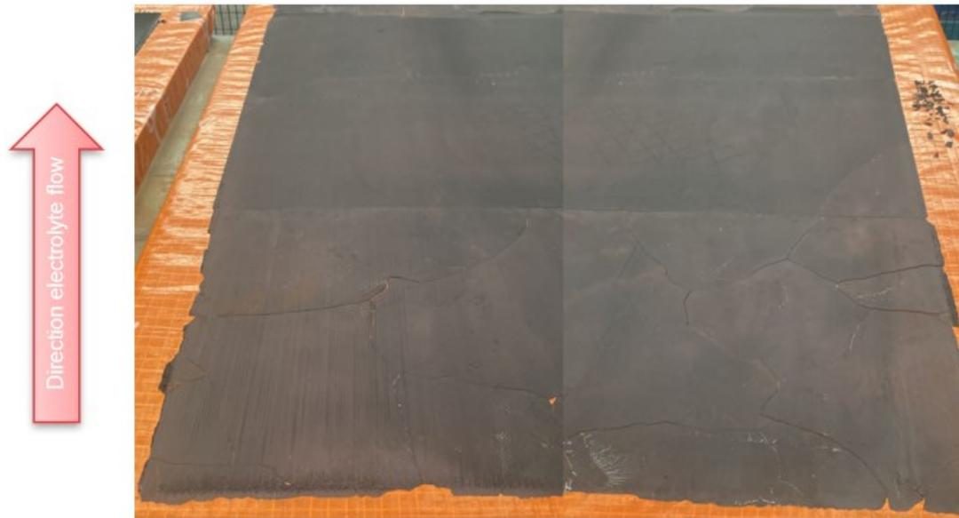
Figure 11: Iron plate produced on the Siderwin pilot with the modifications made on the cell to improve the electrolyte flow.
